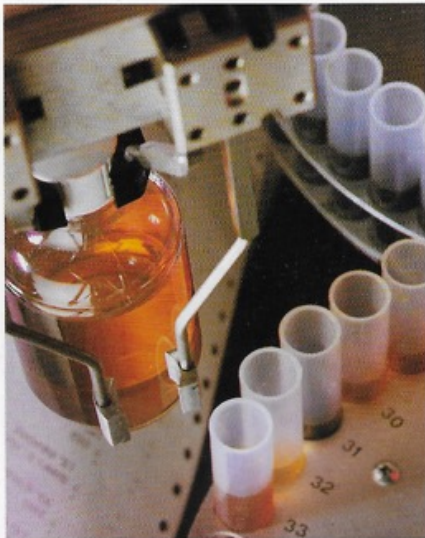
Samples are prepared by robots prior to detailed laboratory testing, as part of Century's Controlled ENGINEERING Tribological (CENT) concept which helps customers get more productivity from critical items of machinery.
