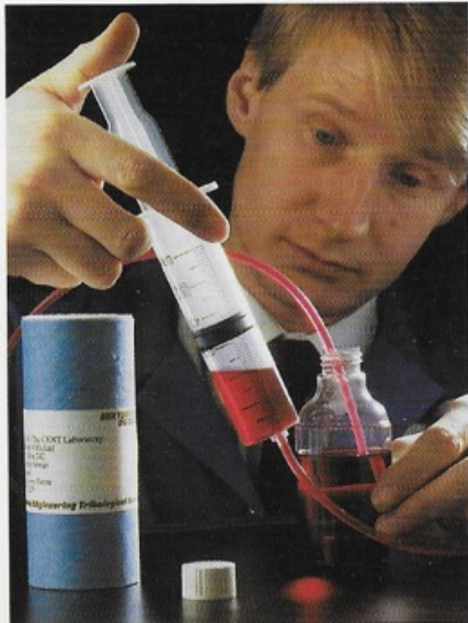
Customers use sampling kits provided by Century to take samples from machinery for analysis by Century's CENT system.
