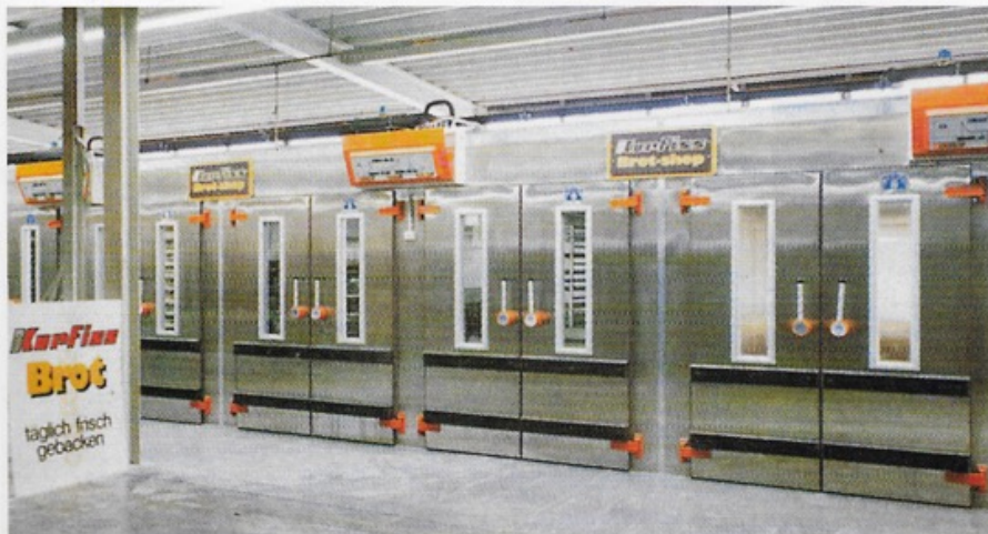
Fully automatic dough conditioning equipment with KOMA's CDS computer-controlled dough controller within a German industrial bakery.
