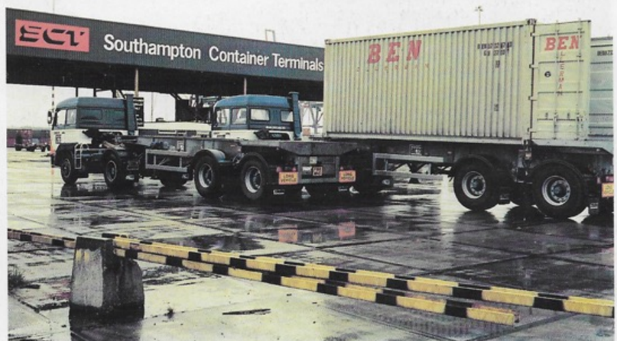
Two of the new lightweight skeletal trailers ordered by ACT Services from Craven Tasker in operation at Southampton Container Terminal. The Ben Line container at right has its doors open and the platform up so that a forklift truck can load from the loading dock.
