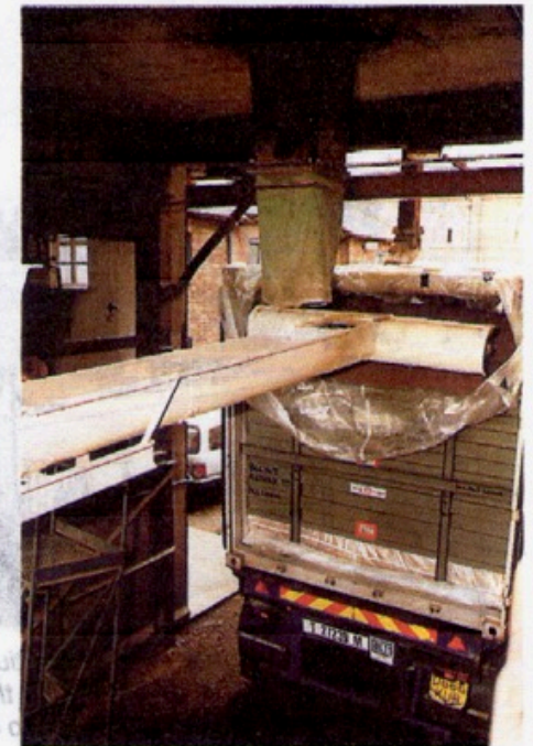
After it has been fitted with the special bulkhead and polythene liner, the container may be loaded by one of a number of different methods — by twin screw conveyor specially trailer mounted (above left), pictured at Pauls Malt Ltd., and by single screw conveyor (at right) with end T-piece spreader, which is taking place at Crisp Malting Ltd.
