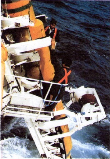
Ready for launching. The torpedo shaped GLORIA is towed behind a ship and emits pulses of sound in a fan-shaped beam on either side at right angles to the ship's track.
