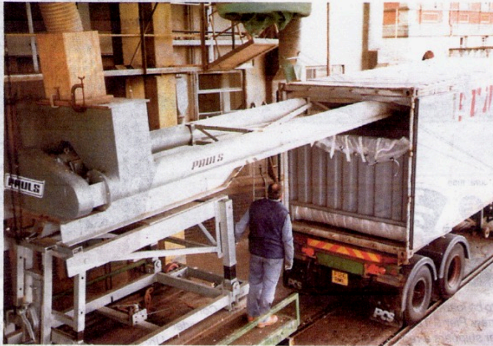
After it has been fitted with the special bulkhead and polythene liner, the container may be loaded by one of a number of different methods — by twin screw conveyor specially trailer mounted (above left), pictured at Pauls Malt Ltd., and by single screw conveyor (at right) with end T-piece spreader, which is taking place at Crisp Malting Ltd.
