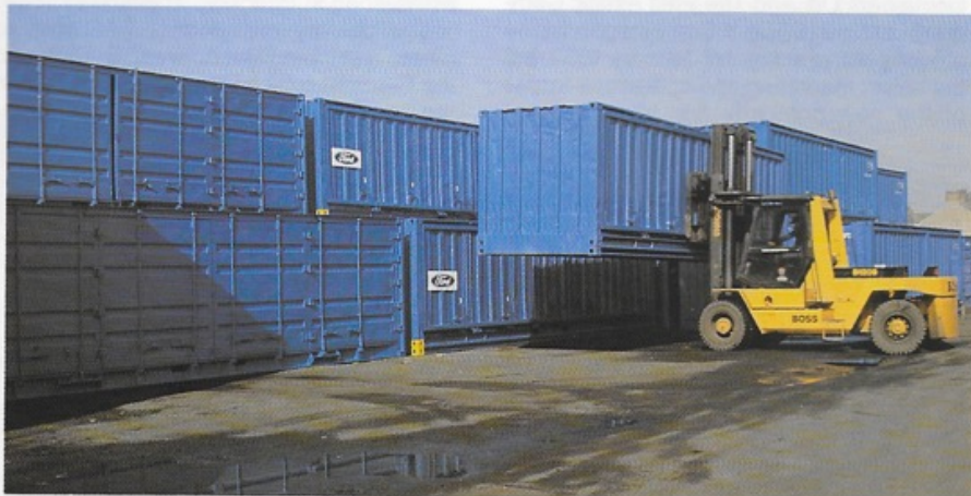
Another refurbished Ford 30-foot ISO container comes from the paint shop at CRL's Dagenham depot, ready to be decaled, have Ford logos fitted and then undergo a final inspection before being delivered to Ford's Dagenham plant.
