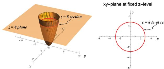
FIGURE 14. The  $z = 8$ -section and  $c = 8$ -level set of  $z = f(x, y) = x^2 + y^2$ .
