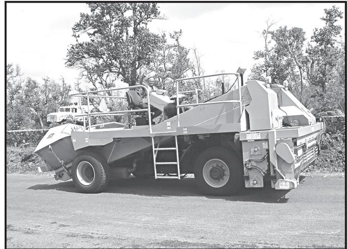
*The new Etnyre Chip Spreader makes our work more accurate and safer for the crew.*
