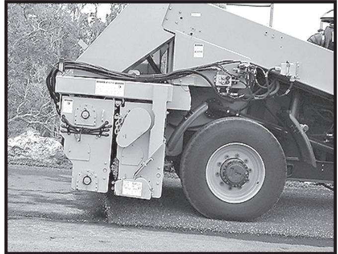
*The spreader drops an even layer of chip into the fresh oil.*
