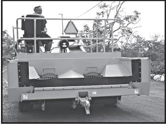
The self-propelled Etnyre Chip Spreader (see photo page 7) has a hitch on the back; it can tow our dump truck, loaded with blue rock chip, without
