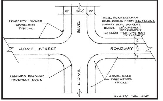
This illustration explains the roadway and easement dimensions on our roads. Please remember that all measurements are made from the center of the actual surveyed roadway. Centerlines may be determined by the pins placed in each intersection. Encroachments cannot be tolerated for safety's sake. If you have questions, please feel free to contact our office by phone, fax or e-mail.
