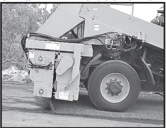
The spreader drops an even layer of chip into the fresh oil.
