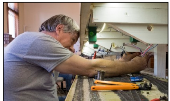
Left, Ray Rumble describes the layout to visitors. Above, Dick Christ solders power drops from the track to the main power bus wires.
