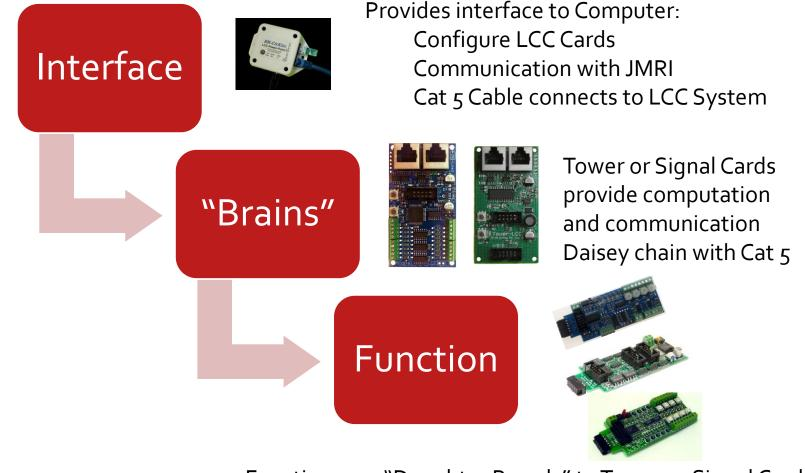
Functions are "Daughter Boards" to Tower or Signal Cards Operate Turnouts, Detect Occupancy, or control discreets Connect with 10 wire flat cable to Tower or Signal Card
