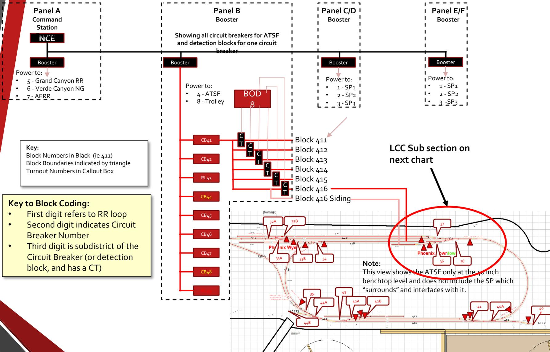
Track Plan of ATSF on 40 inch level showing assigned Block and Turnout Numbers
