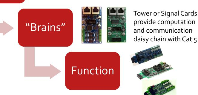
Functions are "Daughter Boards" to Tower or Signal Cards Operate Turnouts, Detect Occupancy, or Auxiliary Equipment
