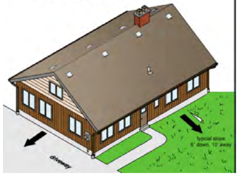
Recommended grading slopes
