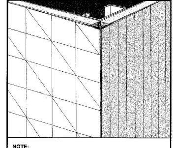
WHEN TUCKING EDGES OF WALLCOVERING INTO CHANNEL. ALWAYS APPLY MASTIC FIRST TO ENSURE THAT PROPER BONDING IS MADE. USE CAUTION NOT TO SCORE OR TEAR EDGES OF WALLCOVERING WHEN TUCKING.
