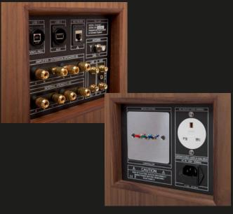
Rear facing input/output panels offer an abundance of pre-wired analogue, digital, RF and filtered mains power interconnectivity as well as mood lighting control. These can be customised and updated at any time to your exacting requirements.
