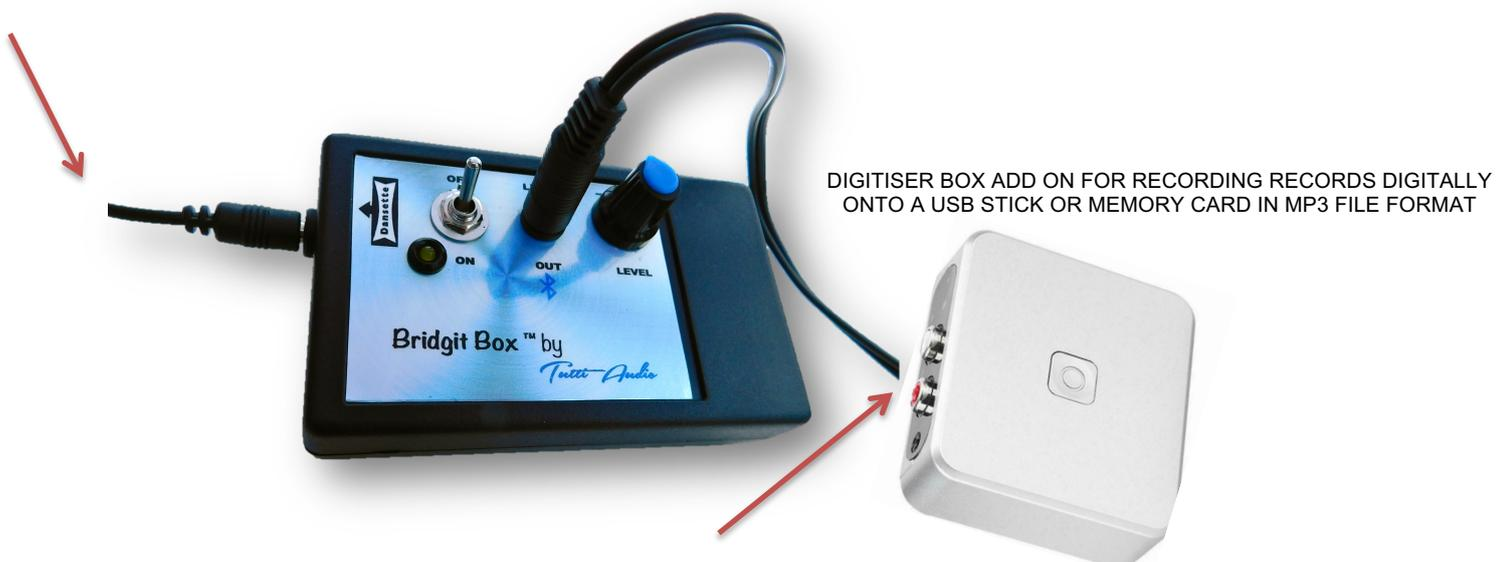
CONNECT TO 'LINE IN' OR 'AUX IN' ON TARGET EQUIPMENT (AMP/HIFI SYSTEM/POWERED SPEAKER OR DIGITISER BOX ETC.)
