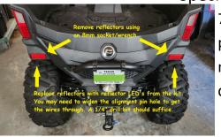
7. Remove the reflectors with an 8mm wrench or ratchet. Replace them with the LED lights that came in your kit. You may need to enlarge the alignment pin hole a little with the 1/4" drill bit to get the wires through.
