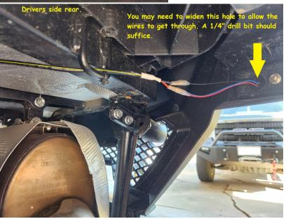
9. On the drivers side. Connect the black wires together. Connect the red/ blue wires to the red wire. Run the crossover cable to the passenger side as indicated in the next photo. Don't zip tie anything until you get done.
