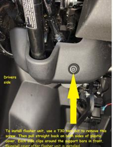
4. If you haven't installed your flasher unit you should do it now. Use a T30 torx bit to remove the screw pictured. Then pull straight back on both sides of the plastic knee guard to unclip it from the support tubes. Installation is the reverse.
