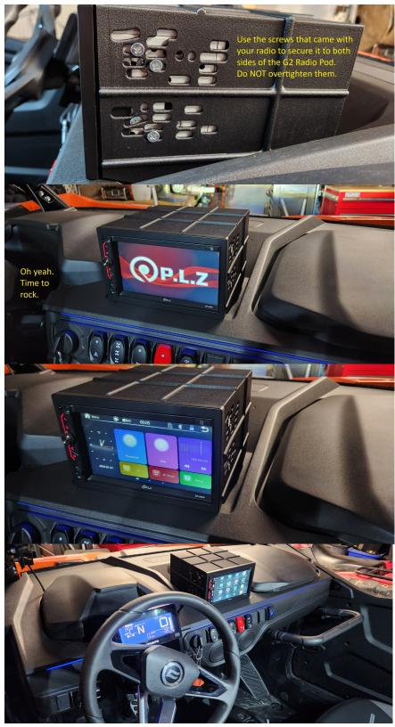
Use the screws that came with your radio to secure it to both sides of the G2 Radio Pod.
