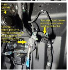
3. Remove the protective cover from the 4 pin plug. It may be clipped to the firewall in your machine. Mine was not. Install your Key On Accessory Point. Push it in till it clicks. Pro tip—apply a little dielectric grease.
