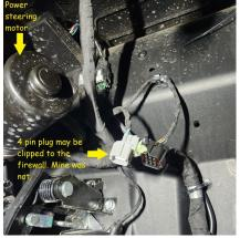
2. Both the 9 pin plug on the right and the 4 ping plug on the left should have protective covers on them to keep dust & water out.
