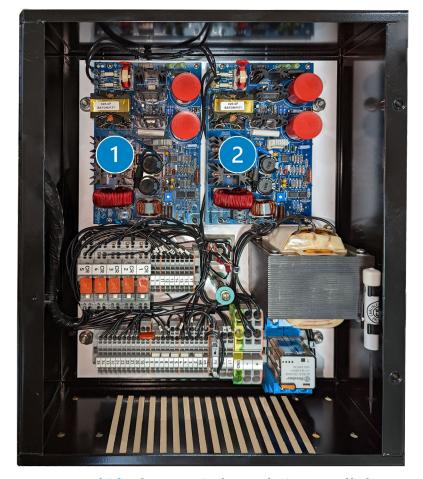
Two (2) electronic boards in parallel provide immediate safety back-up
