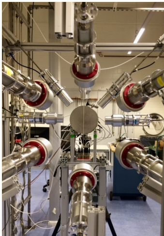
Figure: Illustration of the experimental setup. On the left-hand side, a photo taken from behind the neutron detector arrays is shown. The right-hand side shows a cross-section through the setup, where relevant dimensions are given.
