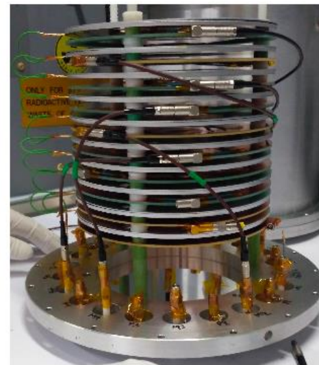
Fig. 23. A setup consisting of ten MicroMegas detectors, coupled with six ^{241}\text{Am} samples and two ^{235}\text{U} and ^{238}\text{U} reference samples, before insertion into the chamber.
