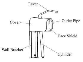
1. Loosen screws and slide aluminum cover forward until it stops against the screws. This action should release the wall bracket, which can be removed by holding on to the cover and pulling the wall bracket downward.
