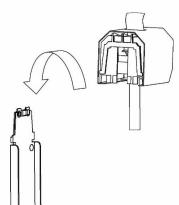
4. Slide the cover back until it touches the wall surface. Tighten the screws located on the underside of cover.
