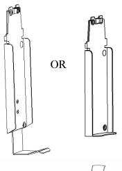
2. Use screws and plugs provided (or other appropriate fasteners) to mount the wall bracket. Allow 11" of space below wall bracket so that the bottle can be removed easily.
