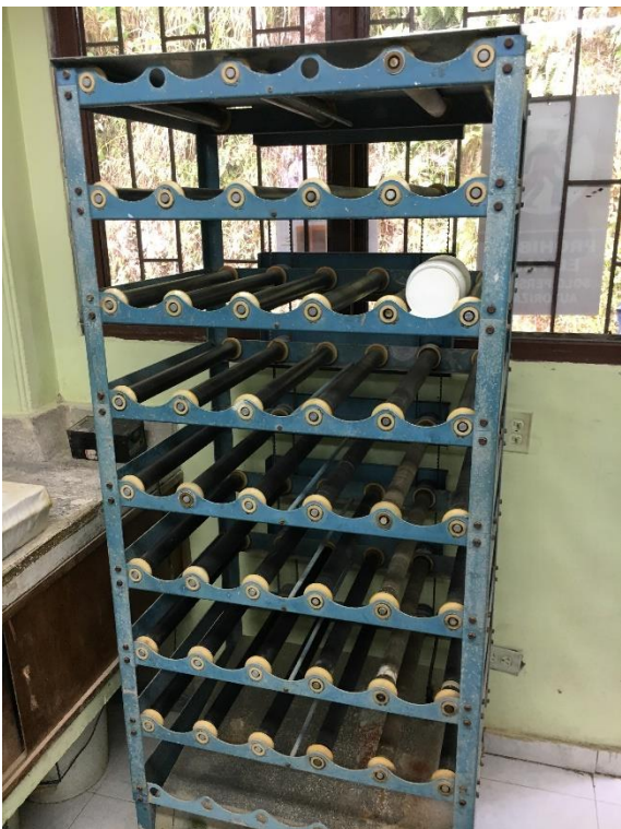
Figure 78. Bottle roller for Leachwell assays.
