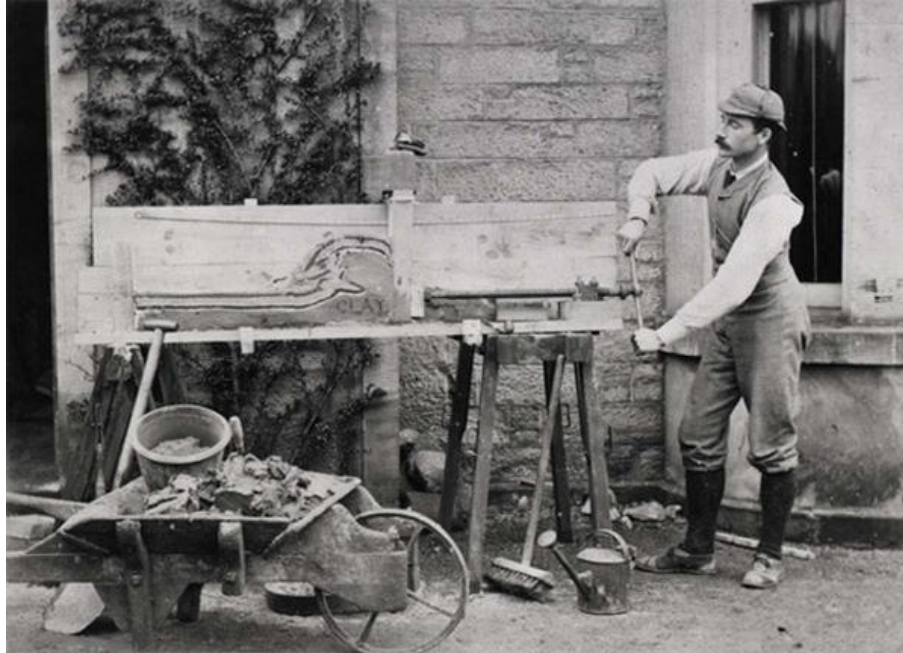
Figure 94. H. M. Cadell's in 1886 turned the handle to move the wall to the left which caused the sand and clay to be compressed.
