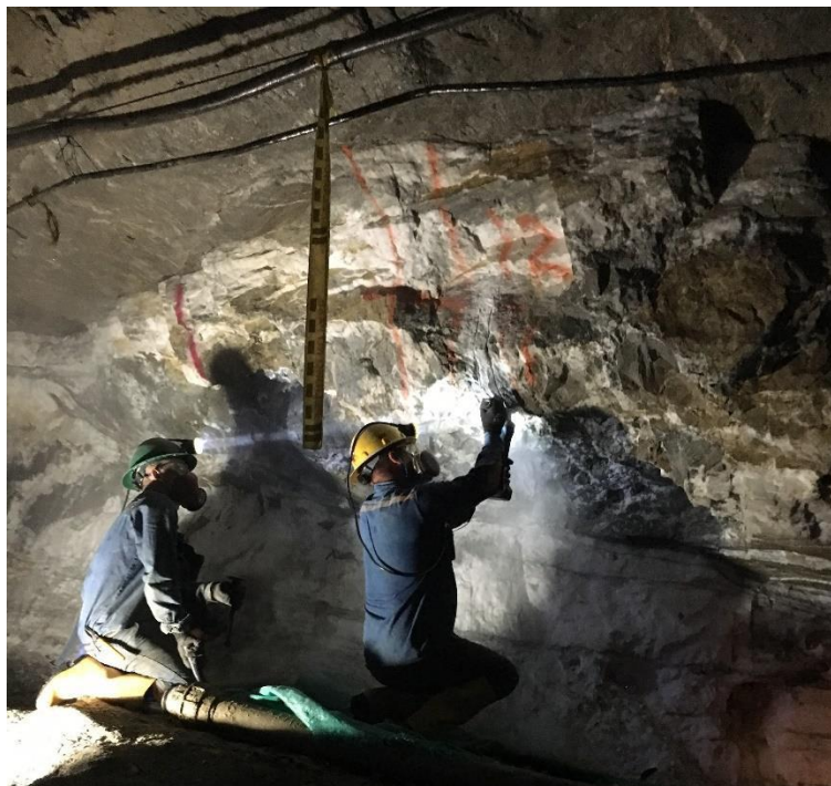
Figure 22. Sampling of the walls inside the mine using an electric saw.
