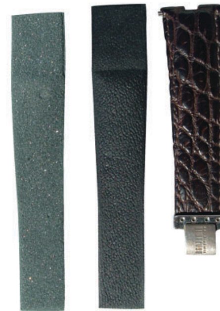
(L-R) Third generation molded polyurethane foam core, skinned foam blank, fifth generation strap assembly.
