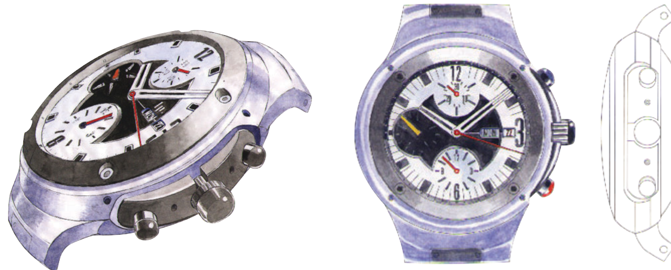
GRANDE CHRONOGRAPH MANTA RAY, 1999: 40mm with active petite seconds subdial. Designed for Valjoux 7750 automatic movement.
