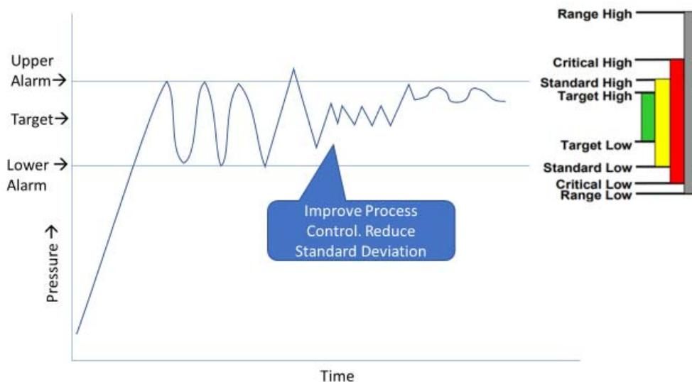
*Applying the Integrity Operating Window concept to Alarms. Note that the Alarms are used to show the edges of important boundaries. These start with the HAZOP.*
