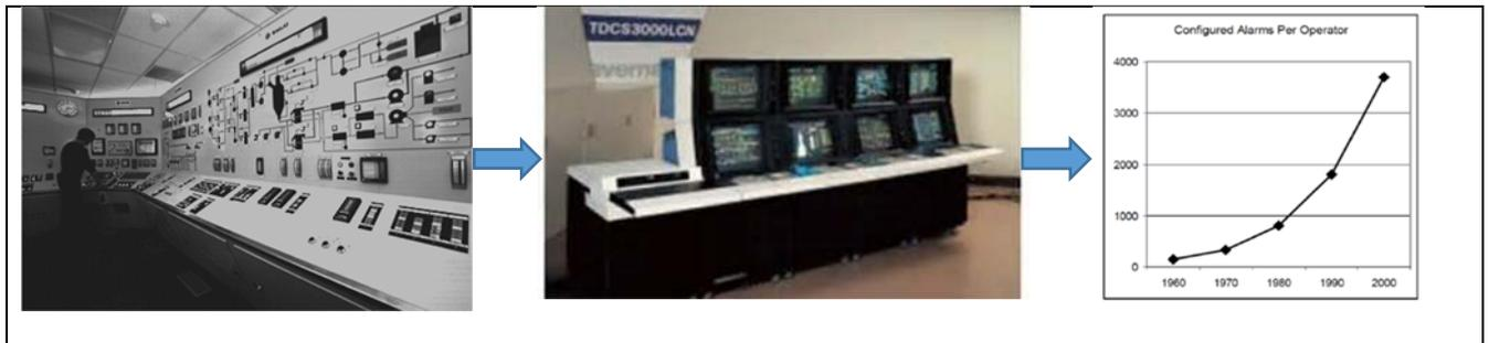
**Figure 1. Evolution of Control System, resulting in rise of alarms per operator**
