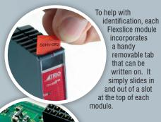
The robust metal chassis provides a good earth from the pcb of each module to the DIN rail to reduce noise and dissipate heat.
