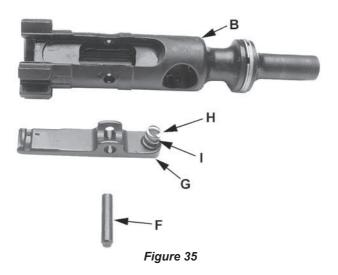
9. Clean bolt and bolt carrier components with a quality gun cleaning solution. Lubricate components with a quality gun lubricant.
