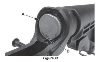
3. Remove the buffer (A) and spring (C). See figure 42.
