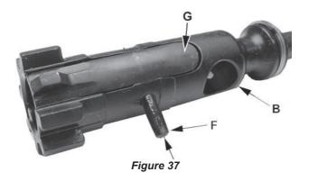
3. Install bolt assembly into bolt carrier. Insert cam pin (D) and turn 90°. The hole in pin will align with the hole through the bolt. See figure 38.
