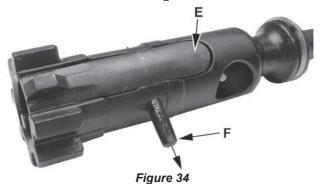
8. Remove extractor pin (F) and extractor (G) from bolt (B). Do not remove insert (I) from extractor spring (H). See figure 35.
