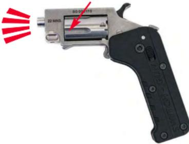
When firing the Switch Gun<sup>®</sup>, be sure all persons are a safe distance to the rear of the shooter. When fired, all revolvers discharge hot gas and particles of lead, powder grains, or lubricant through the clearance gap between the cylinder and the rear of the barrel. These high-speed discharges can injure a person who is standing too close to the revolver.
