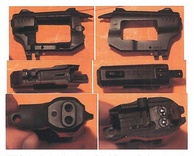
FTISB found that the submitted sample has a cylinder similar to a revolver that must have each chamber manually loaded prior to firing and spent cases manually ejected.
