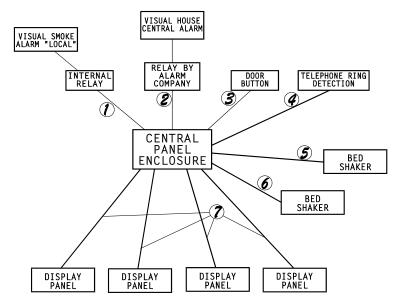
Figure 2.1 - System Block Diagram
