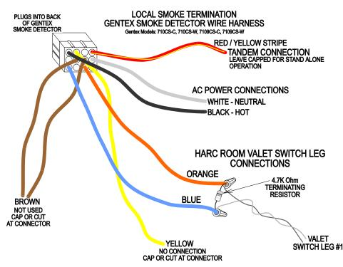
Figure 3.16 - Gentex 710cs Wiring Harness W/ Valet Connections
