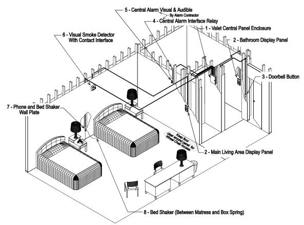
Figure 1.1 - Valet Component Layout in a Typical Room
