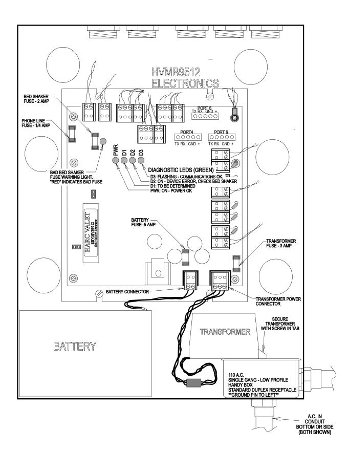
Figure 3.20 - Central Panel Enclosure Main Power Wiring
