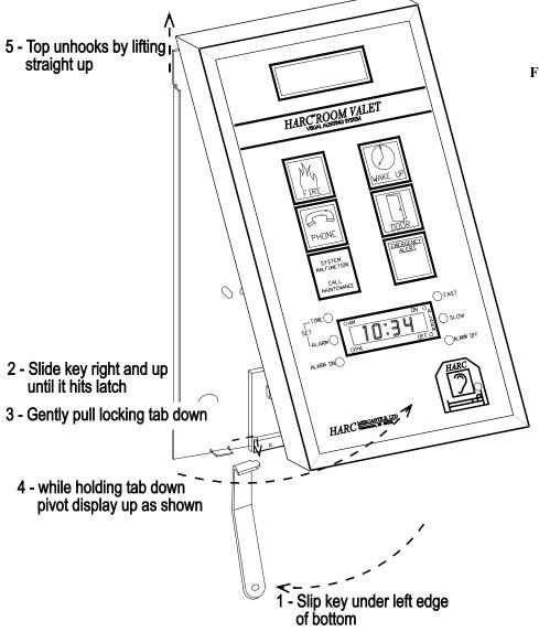
Figure 3.2 - Unlatching the Valet Display Panel
