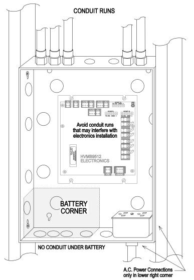
Figure 2.8 - Central Panel Enclosure Conduit Locations
