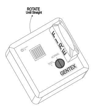
Figure 3. 18 - Installing a Gentex Smoke Detector Onto it's Mounting Bracket
