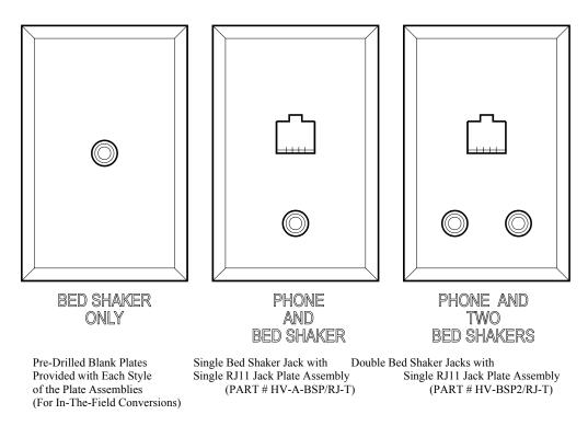
Figure 3.13 - Bed Shaker(s) Jack and RJ11 Jack Wall Plate Assemblies
