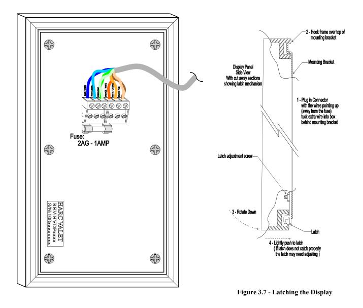
Figure 3.6 - Back View of Display Panel showing connection
