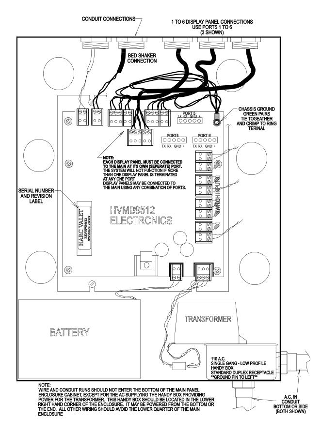
Figure 3.10 - Central Panel Enclosure Main Electronics Output Terminations
