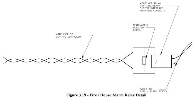
A Installation Hint: All switch legs are terminated at the switch end with a 4.7 KOhm resistor. Any 4.7K Ohm, 5% tolerance, 1/4 Watt or 1/2 Watt resistor will work.
