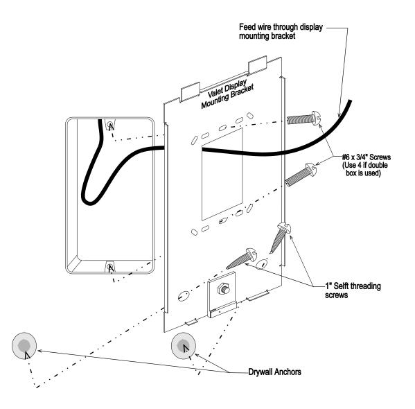
Figure 3.3 - Installing a Display Mounting Plate
