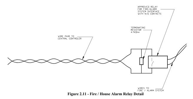
A Installation Hint: All switch legs are terminated at the switch end with a 4.7K Ohm resistor. Any 4.7K Ohm, 5% tolerance, 1/4-Watt or 1/2-Watt resistor will work.
