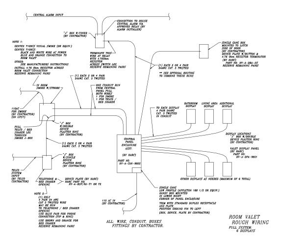
Figure 2.4 - Valet Rough Wiring Layout
