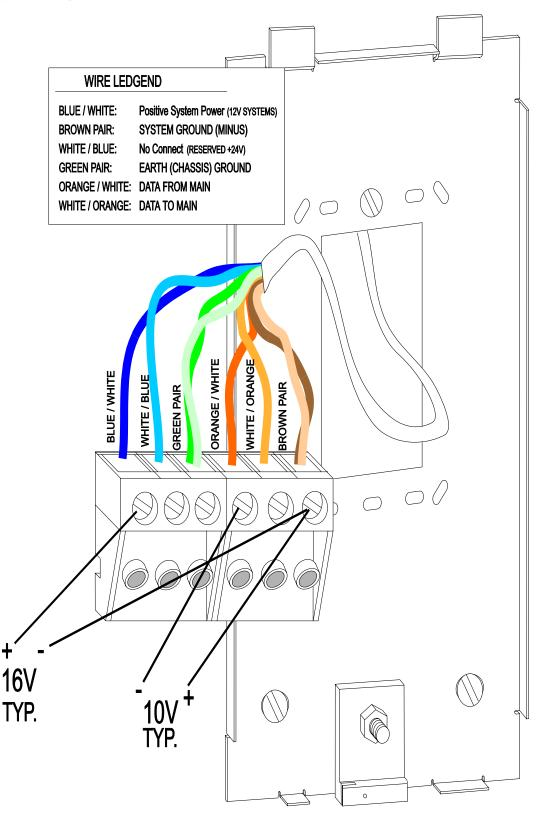
Figure 3.5 - Typical Voltages on the Display Panel Connector
