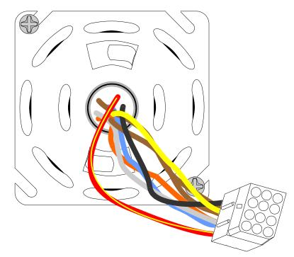
Figure 3. 17 - Gentex Mounting Bracket Ready for Detector
