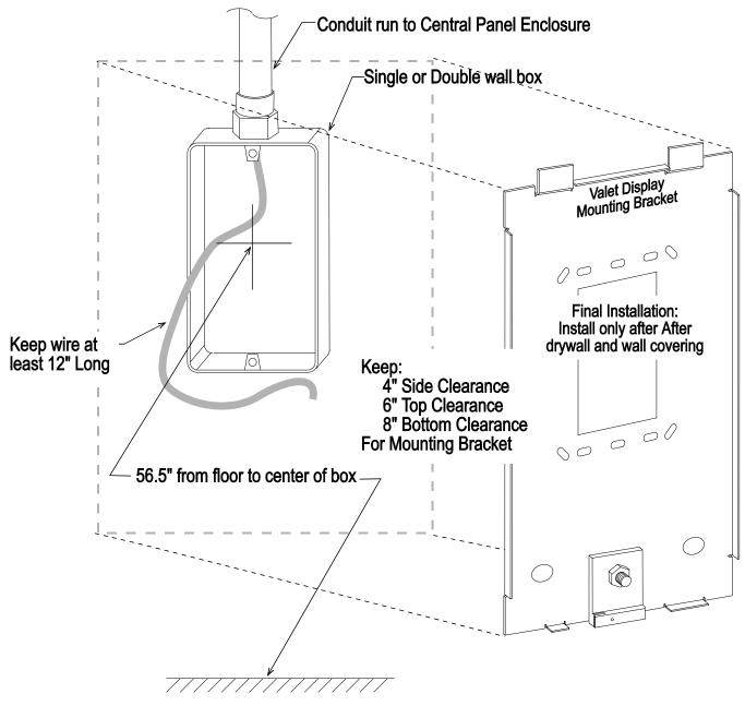
Figure 2.9 - Display Panel Rough install
