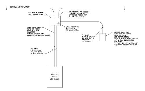
Figure 2.5 - Rough Wiring Combined Door Button and Central Alarm
