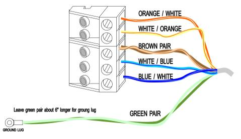
Figure 3.9 - Processor Port Wiring (Recommended Colors)
