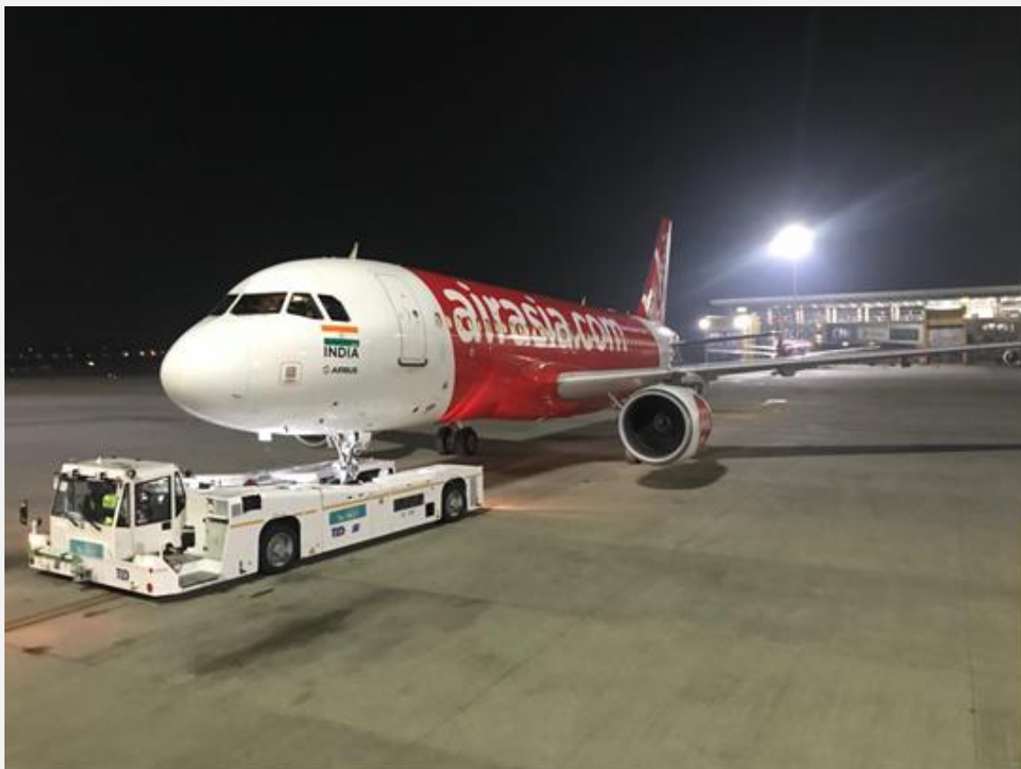
Photo courtesy of Alternate Aeroworks Canada Inc. A TaxiBot connected to an Airbus aircraft
