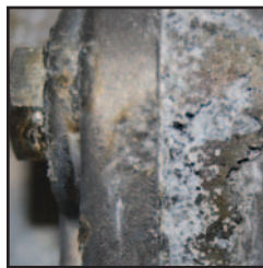
Corrosion of a Nickel Teflon coating after salt spray testing.
