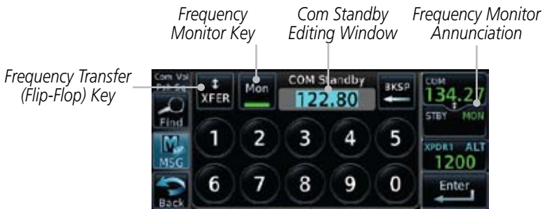
Figure 3-21 Com Frequency Monitoring
