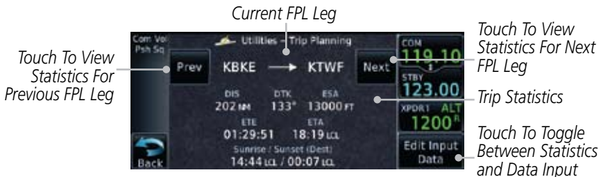
14-26 Utility Trip Planning Page Computed Data View Of Next Waypoint (Flight Plan Mode)
