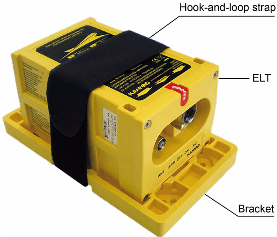
Figure 6: INTEGRA ELT with Mounting Bracket P/N S1840502-02
