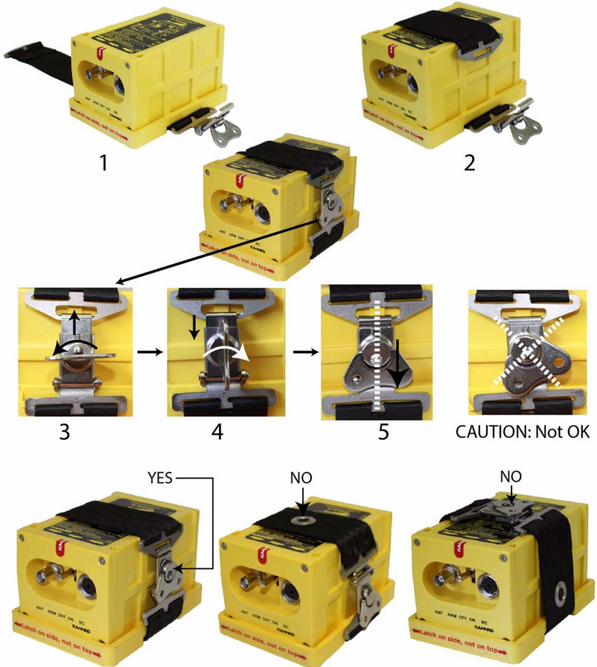
Figure 204: ELT installation with Mounting Bracket INTEGRA AF P/N S1850551-04
