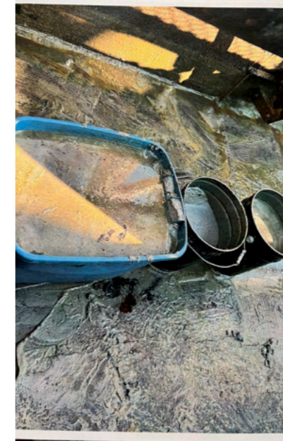
Silty sand filtered by the Hydrocyclone
