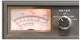
Note from the editor: ZeroBeat has received several correct answers to the quiz regarding d"Arsonval movements. Yes, d'Arsonval movements are involved in the traditional design of meters, with the d'Arsonval principle used to move the meter needles.
