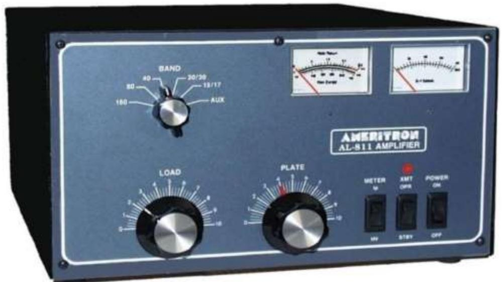
The Ameritron AL-811, one of the most popular amplifiers around. It puts out about 600 watts with three 811 tubes. It was so popular because it could be run on 110v AC home current. Many amplifiers require 220v. As you can see, these tube amplifiers have LOAD and PLATE controls that require tuning up before operation on a frequency. There are solid-state no-tune amplifiers on the market. They are more expensive.
