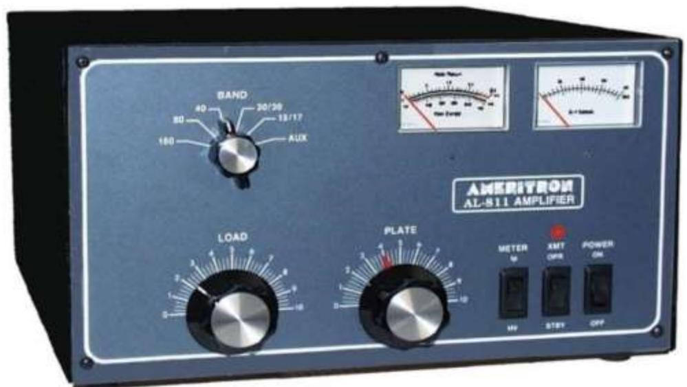
The Ameritron AL-811, one of the most popular amplifiers around. It puts out about 600 watts with three 811 tubes. It was so popular because it could be run on 110v AC home current. Many amplifiers require 220v. As you can see, these tube amplifiers have LOAD and PLATE controls that require tuning up before operation on a frequency. There are solid-state no-tune amplifiers on the market. They are more expensive.
