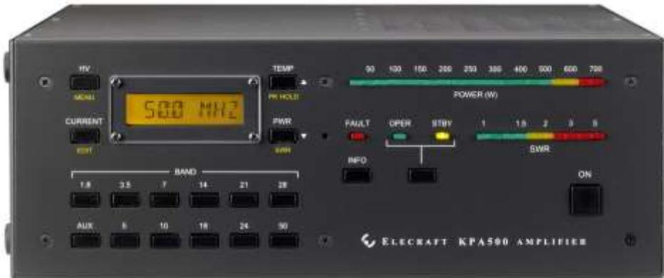
The Elecraft KPA-500 is an example of a modern solid-state no-tune 500-watt amplifier. It senses the RF from your transceiver and decides which band is being used. This amplifier runs \$ 2,799.85 before tax and shipping. It is easy to operate but is very sensitive to your SWR. An SWR of 1:2 or higher will trip a protective circuit.
