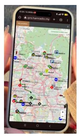
In addition to the well-known position reports from vehicles, APRS is used to send reports from unattended weather stations, announcements of events like ham fests and swaps, coordinate search-and rescue efforts, etc. APRS can also exchange short one-liner cellphone-style-SMS text messages between specific callsigns, and even to/from internet email addresses.
