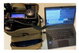
Because of VARA's incredible weak-signal capability, it is practical for a mobile or RVer to be tracked and to communicate almost anywhere with low power and modest antennas, i.e. Yaesu FT-818 "porta-luggie" and a 30M HamStick-type whip or random wire. During my 6300-mile round-trip from central Michigan to Los Angeles and back this October, my mobile was being heard and gated to the Internet almost constantly using a FT-891 transceiver with
