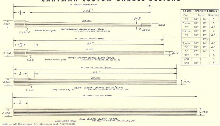
All are new barrels made from Timken gun barrel quality, electric furnace, chromemoly alloy steel specially heat-treated and stress relieved. Barrels are approximately one inch longer than standard for working purposes. This amount must be cut from the muzzle at final finishing to insure uniform bore diameter and maximum accuracy.
