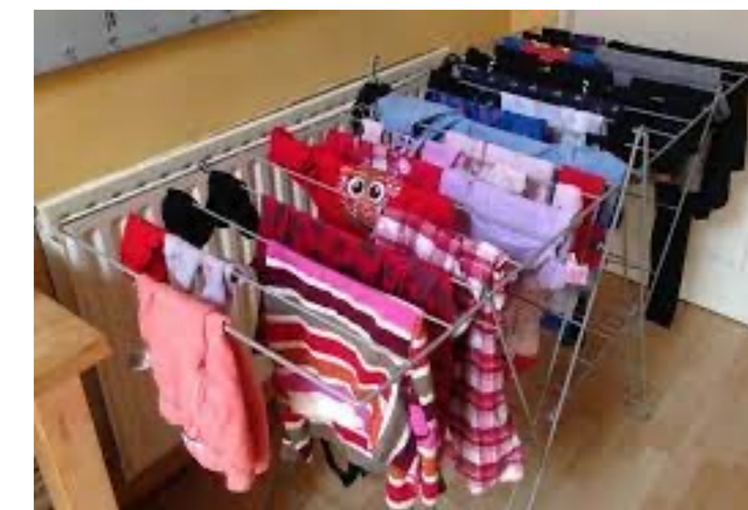
Damp and Mould – Drying clothes in a poorly ventilated space leads to a buildup of condensation.
