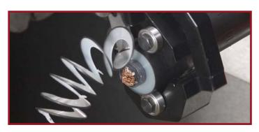
Knife "A" for stripping main insulation layer.
