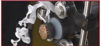
A single blade can strip both semi-con and main insulation layer of the cable. Chamfering at the same time.
