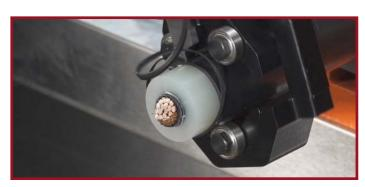
• Knife "B" for stripping non-peelable semiconductor layer.
