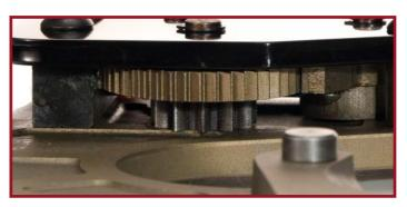
• Die-forged driving gears can bear stronger cutting resistence while saving labor.
