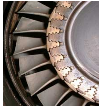
Figure 2: Example of Turbine Blade 'fir-tree' Attachment
