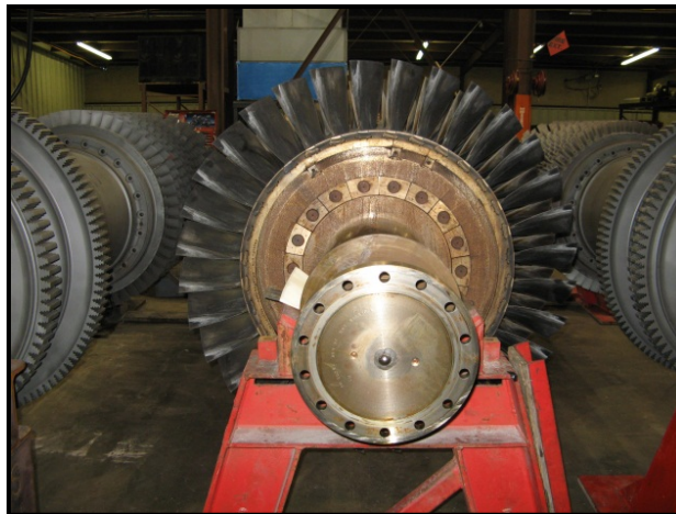
Figure 2. Rotor of GE 5002 Gas Turbine Prior to Overhaul
