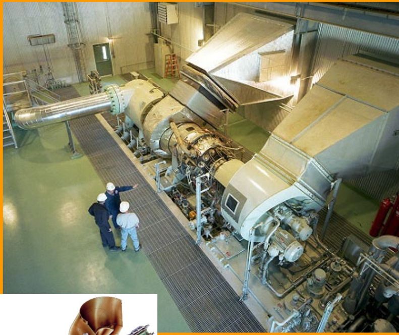
2-shaft gas turbine
