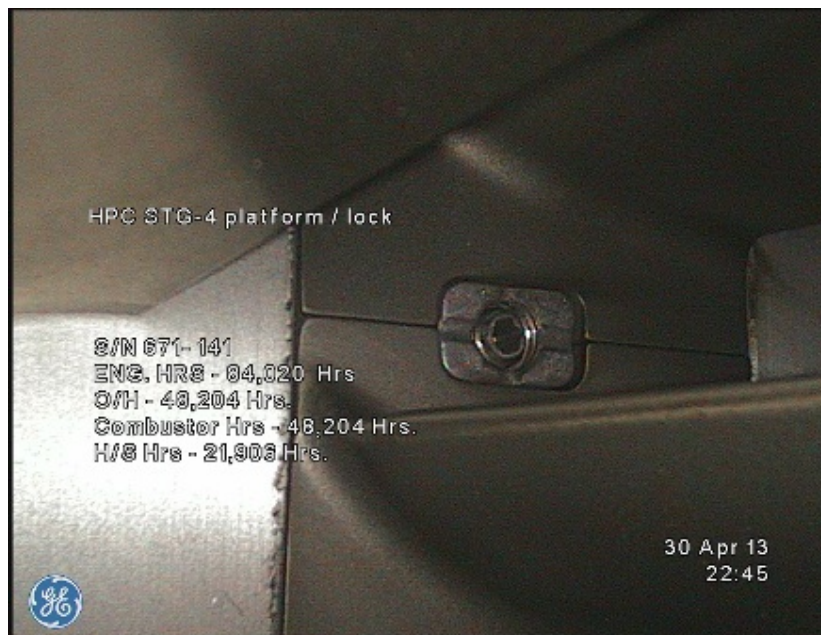
Figure 14 – Kerrobert HPC Stage 4 after 21,906 hours operation with HEPA filters and no water washes
