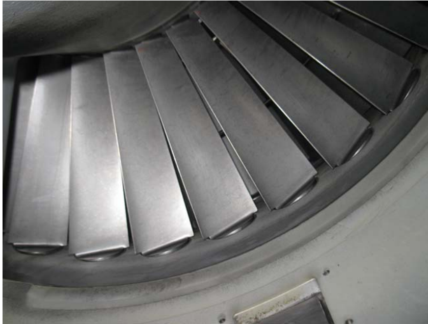
Figure 13 - Kerrobert Inlet Guide Vanes (IGV) after 21,906 hours operation with HEPA filters and no water washes
