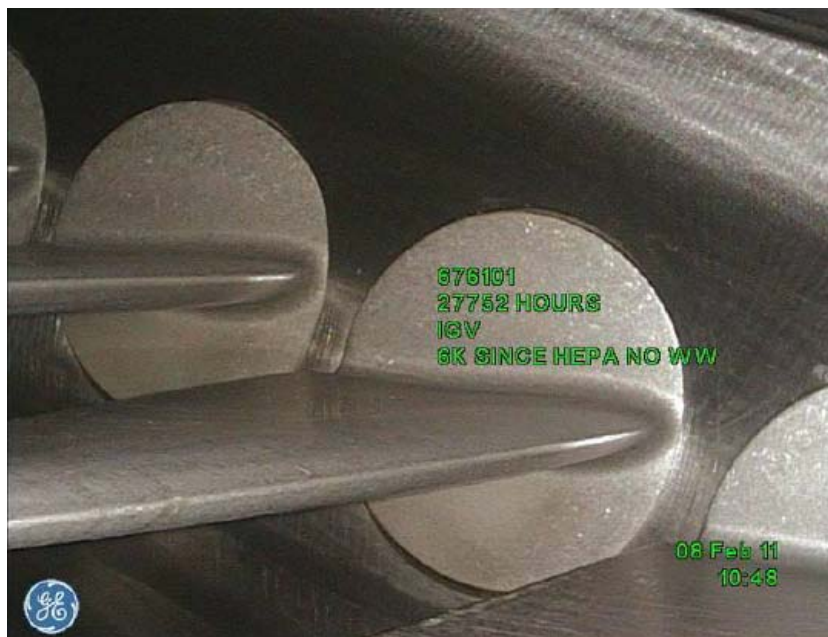
Figure 10 - IGV after 6000 hours with no water wash
