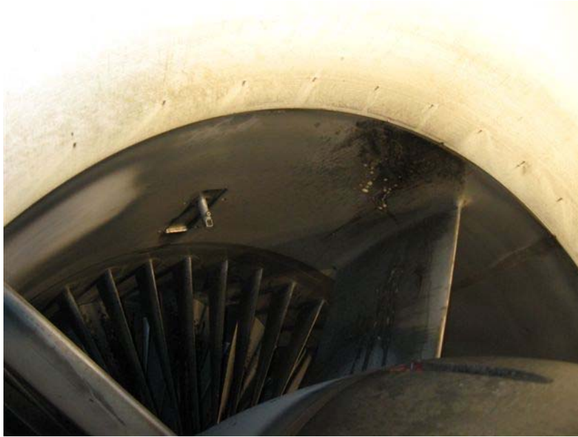
Figure 2 – Dirt & fouling on front frame and Inlet Guide Vanes (IGV) on an Alliance Unit
