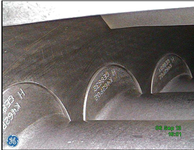
Figure 11 – Windfall Stage 2 Variable Stator Vanes outer bearing, 2.5 years (18,450 hours) after previous OWW and inspection
