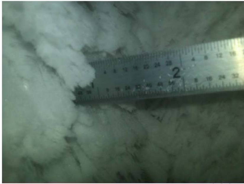
Figure 16- Hoar frost build up on LM2500 turbine inlet filters at Wimbledon Pumping Station
