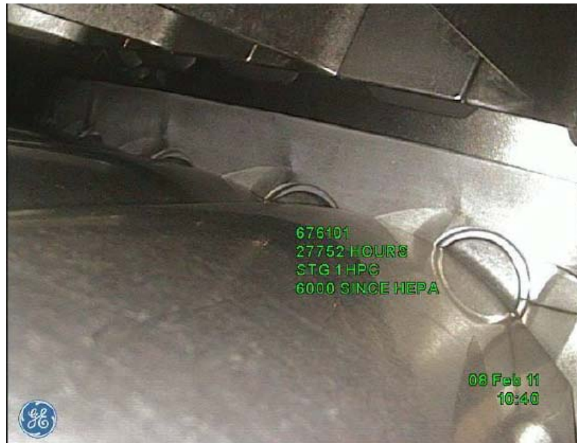
Figure 9 – Stage 1 HPC after 6000 hours with no water wash
