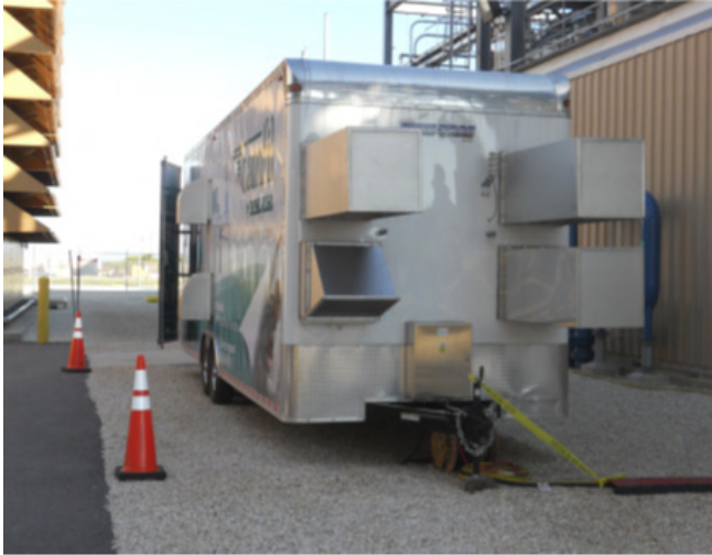
Figure 9: Mobile air filter test laboratory
