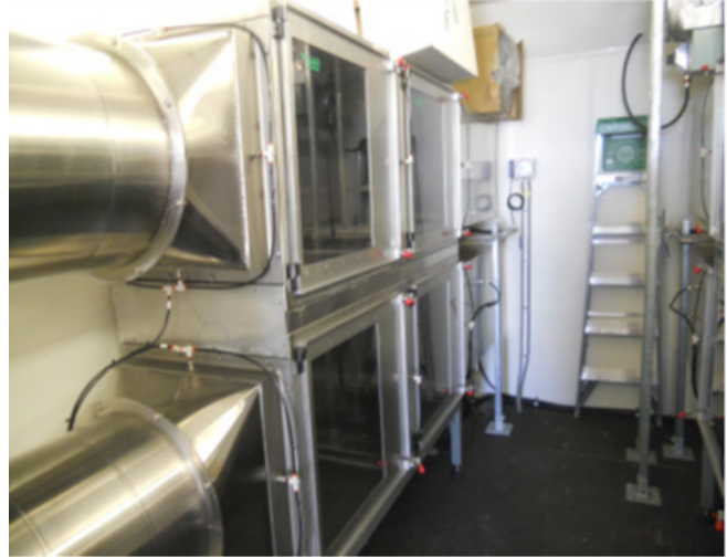
Figure 10: Mobile air filter test laboratory
