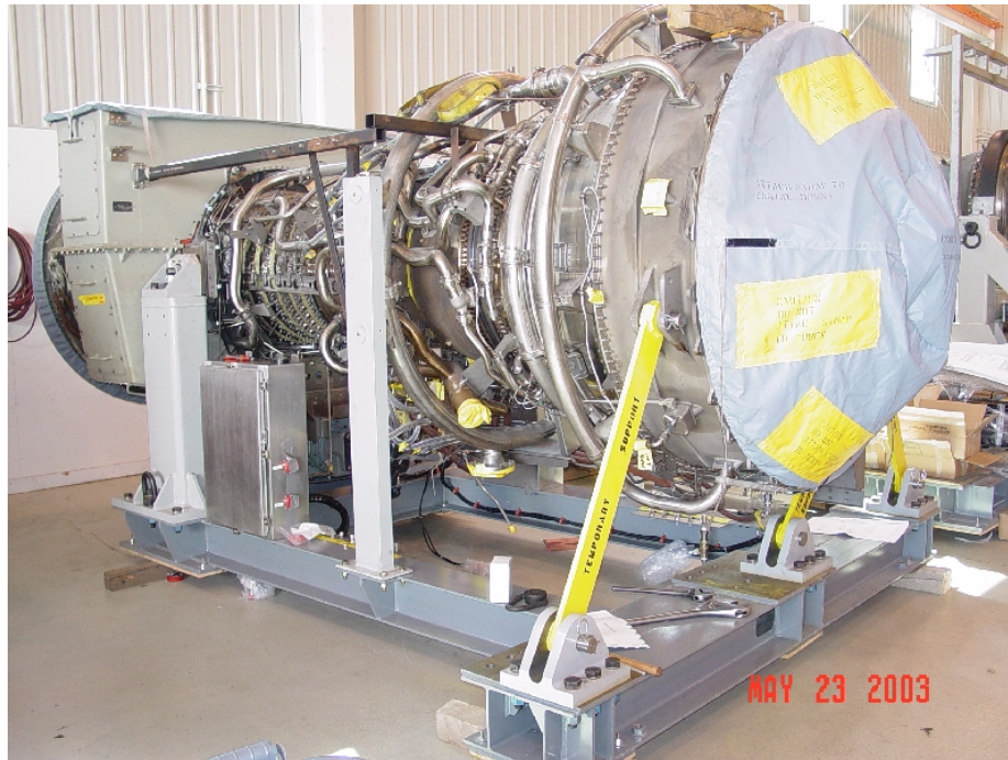
Figure 5 - PC Engine on skid
