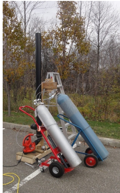
Ambient temperature mock-up exhaust stack and gas bottles
